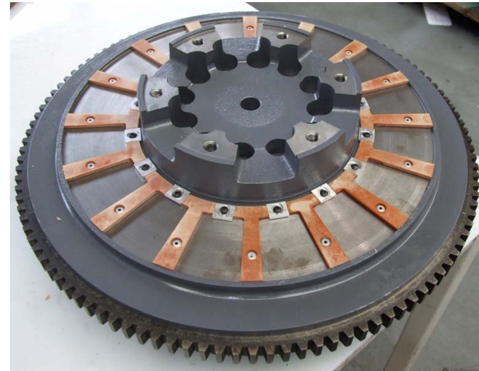
Half of Rotor Assembly showing magnet mounting details
